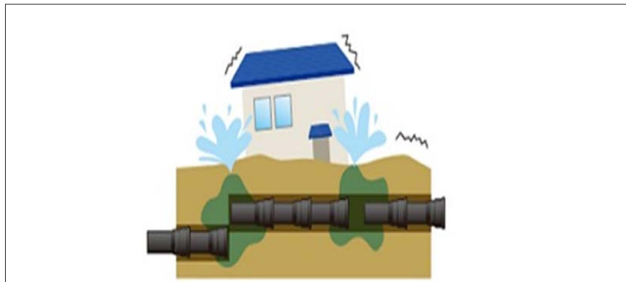
FIG. 7 Example of joint separation.
