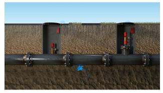
• Leaks can be detected via acoustic correlation and using single sensor assessment.
