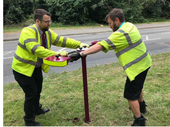
FIG. 1 The UnJammer can be operated by one operator, or if more kinetic energy is required, a second operator can assist.
