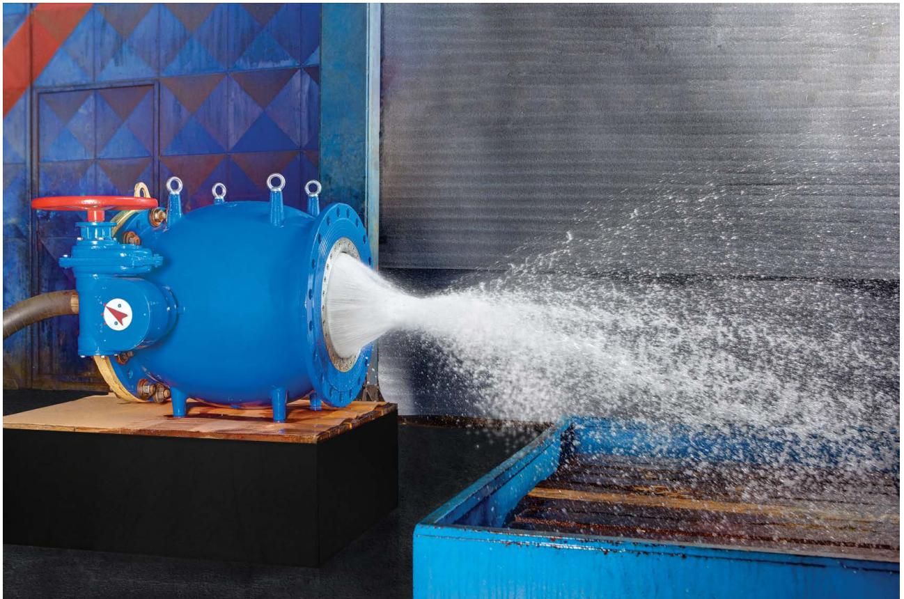
FIG. 13 Converging water streams concentrate vapour bubbles in the centre of the flow to limit cavitation damage and dissipate energy
